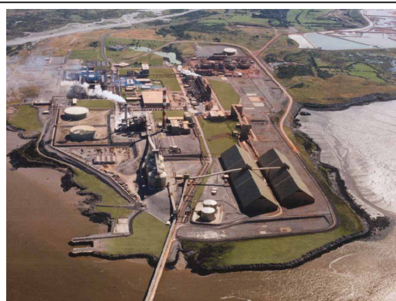
Photo 4: Aerial view of Aughinish Alumina site. The red and white chimney at the CHP plant is seen in the centre of the site.
